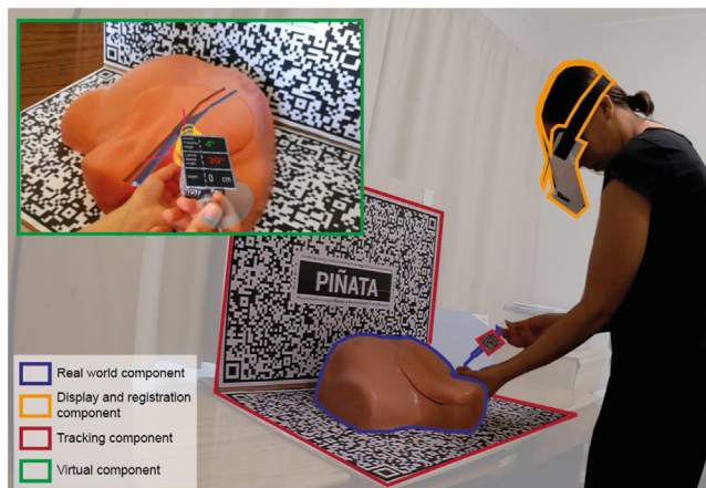
Fig. 3. Overview of the PIÑATA components highlighted in different line colours: real world component (blue lining), registration and display component (orange lining), tracking component (red lining), and first-person view of the virtual component (green lining). (For interpretation of the references to colour in this figure legend, the reader is referred to the web version of this article).
